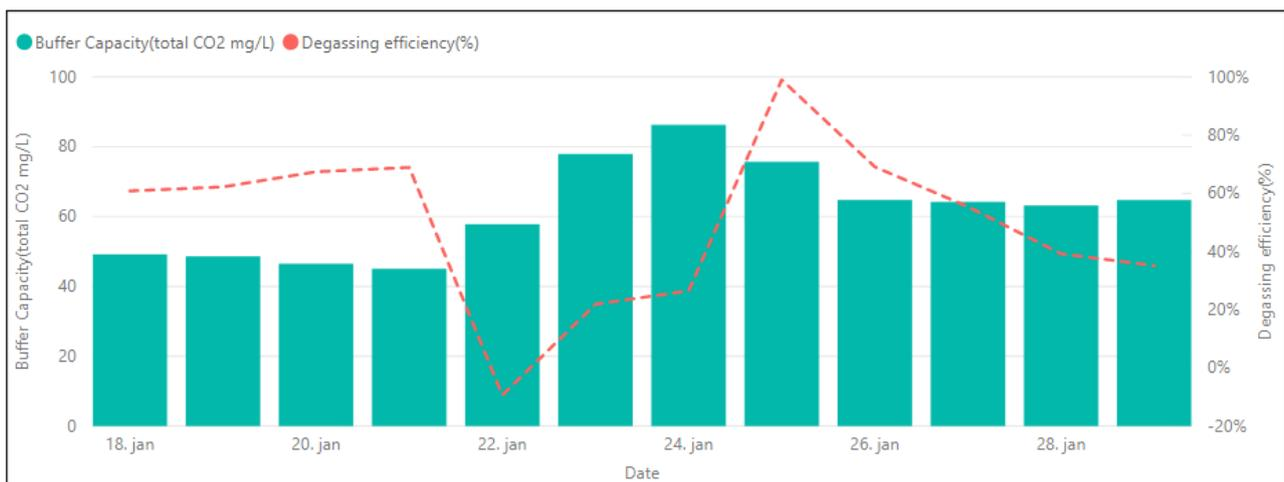
Figure 1 The green bars are the buffer capacity measured as Total CO<sub>2</sub> in mg/L. The dotted red line is the degassing efficiency.
